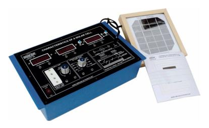
OMEGA TYPE ES-290 Experimental Set-Up has been designed specifically to study the characteristics of a Solar Cell. The set up consists of board with intensity controller, mounted solar cell, table lamp 100W and five different area choppers.
