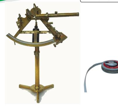
**OMEGA TYPE ES-291** Experimental Set-Up has been designed specifically to determine the height of a distant tower or a building with the help of a Sextant. The set-up consists of a Sextant Stand & Inch tape.
