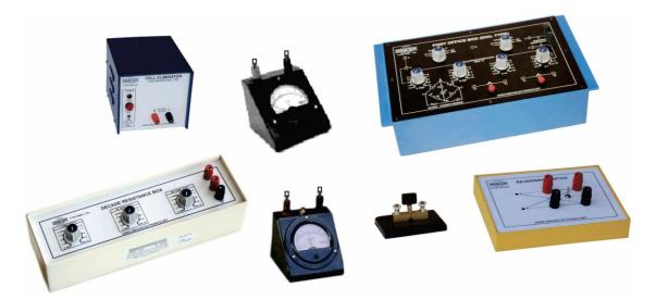
OMEGA TYPE ES-292 Experimental Set-Up has been designed specifically to determine resistance & current sensitivity of moving coil galvanometer by Kelvin's method using Post Office box. The set-up consists of Post Office Box, Galvanometer, Decade resistance box, Leclanche cell, D.C. voltmeter, Reversing switch, Plug key, etc.
