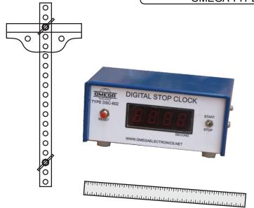
OMEGA TYPE ES-294 Experimental Set-Up has been designed specifically to determine the value of 'g' acceleration due to gravity at a certain place, with the help of a Bar Pendulum.
