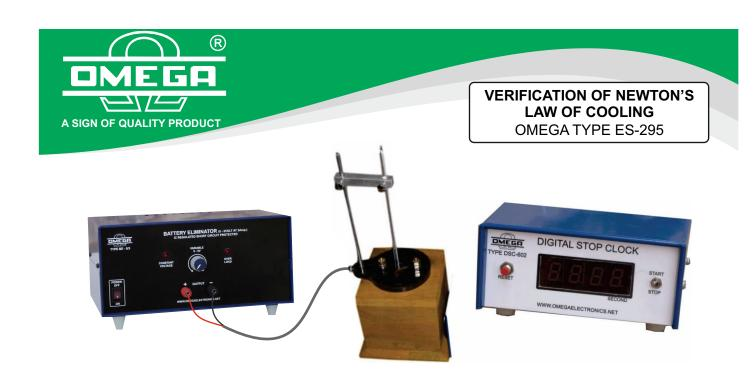
OMEGA TYPE ES-295 Experimental Set-Up has been designed specifically to verify Newton's law of cooling by drawing a coolong curve for the liquid.
