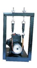
**OMEGA TYPE 20110** Swinburnes Test of DC Machine is an important training system for Electrical Laboratories. It can be aptly employed for understanding the fundamental concepts and functioning of DC Motor. Swinburnes Test is the method through which losses are measured separately and efficiency at any desired load can be predetermined.
