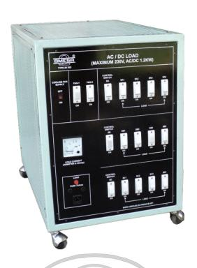
OMEGA TYPE 202 AC/DC Load is an important device in all the Electrical laboratories. One can connect a load upto 1.2KW using this product. The device comes with On Board Switches, so that one can vary the load as required, in steps of 100W. The product is designed so as to provide load for various experiments of Transformer, Motors, Generators etc.
