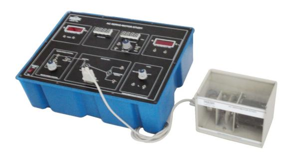
OMEGA TYPE ICT-919 is designed to study Two phase A.C. servomotor which very important electromechanical actuators having applications in the area of control systems. The study of its operating principle and features from a part of the first course on automatic control systems in electrical engineering curriculum. It's small size, low inertia and almost noise and frictionless operation makes the A.C. servomotor particularly attractive in aircraft and spacecraft applications.
