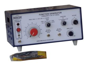
OMEGA TYPE FG-321 Function Generator has been designed specifically to provide a variety of waveforms over a wide frequency range. This versatile instrument is intended to be useful as general purpose signal source in every laboratory work. This generator is based on XR-2206 monolithic Function Generator integrated circuit. It is capable of producing high quality sine, square and triangular waveforms of high stability and accuracy.
