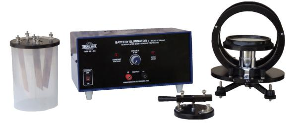
**OMEGATYPE ES-360** Experimental Set-up has been designed specifically to determine E.C.E. of copper and reduction factor of a Helmholtz galvanometer. The set-up consists of Copper Voltameter, Helmholtz Galvanometer, Battery eliminator, Reversing key etc.
