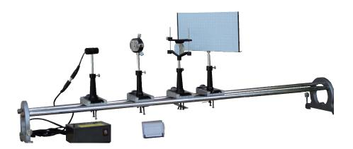
**OMEGA TYPE ES-361** Experimental Set-up has been designed specifically to determine the wavelength of the laser using grating and to determine the slit width. The set-up consist of an Optical bench, Diode laser, Optical screen, Double convex lens, Slit, Diffraction grating etc.
