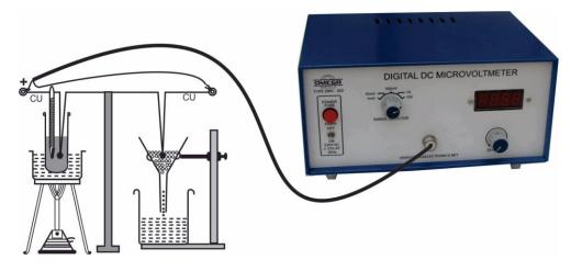
**OMEGA TYPE ES-362** Experimental Set Up has been designed specifically for the study of Different Thermo E.M.F. The aims are to plot thermo emf versus temperature graph and to find the melting point of Paraffin Wax using digital D.C. microvoltmeter and sand bath.
