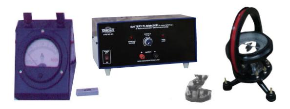
OMEGA TYPE ES-363 Experimental Set-up has been designed specifically to study the variation of magnetic field intensity with the current along the center of current carrying coil.
