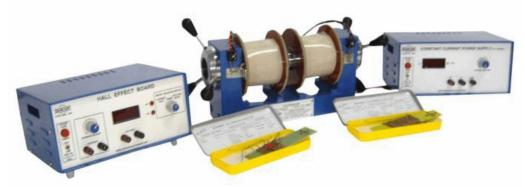
**OMEGA TYPE ES-365** Experimental Set Up has been designed specifically for identification of charge type by hall voltage measurement. The set-up consists of Hall Effect Board, Hall Probe, Electromagnet, Constant Current Power supply (0-4A), and hall probe stand. The set up is complete in all respect and requires no other apparatus.
