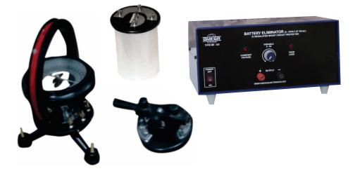
**OMEGA TYPE ES-366** Experimental Set Up has been designed specifically to determine Reduction factor of a Tangent Galvanometer by using copper voltameter. The set up consists of copper voltameter, Tengent Galvanometer, Battery eliminator, Reversing key, etc.
