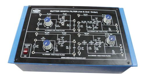
OMEGA TYPE ETB-249 Experimental Training Board has been designed specifically to study. First & Second order of Low Pass Butterworth Filter for a higher cut off frequency of 1 KHz with a pass band gain of 2 & First & Second Order High Butter worth filter for Lower cut off frequency of 1 KHz with a pass band gain of 2.
