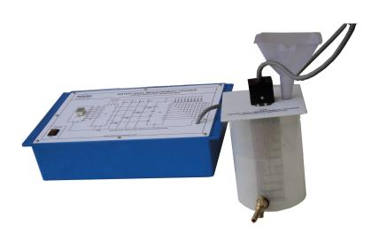
OMEGA TYPE ICT-924 provides study of Water Level Measurement Technique using Inductive Transducer. Water Level Measurement Trainer is designed to learn concept of Water Level Measurement. It helps students & industry professionals to understand operation of level sensors in detail providing the theoretical and experimental knowledge of Inductive Water Level Sensor.
