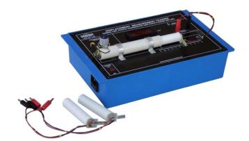
OMEGA TYPE ICT-926 provides displacement Measurement Trainer using LDR, Photo transistor and Photo diode set up & study of their characteristics. The characteristics include Displacement vs Resistance at constant voltage and voltage vs resistance at constant displacement. Different test points are also provided on the panel to facilitate the student to understand without any operation instruction by third person.
