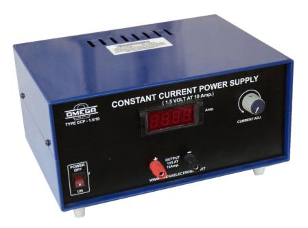
OMEGA TYPE CCP-1.5/10 is a high performance constant current power supply. The current regulation is IC controlled and hence result in the highest quality of performance. Matched Power Transistors are used to share the load current. The supply is protected against transient caused by the inductive load of the magnet.
