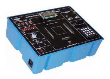
ARM 7 Development Board OE-5004 is a 32-bit development platform and serves as a means for code development. This trainer is designed for students to explore ARM architecture and on board supporting peripherals which provide an ideal platform for extensive embedded development. This trainer provides both the serial and USB connections which can be used to download and run a code on any standard IDE. This trainer allows users to evaluate, prototype and create application specific designs.
