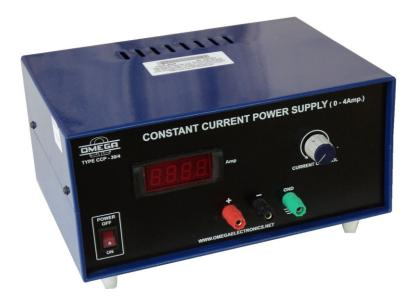
**OMEGA TYPE CCP-30/4** is a high performance constant current power supply. The current regulation is IC controlled and hence result in the highest quality of performance. Matched Power Transistors are used to share the load current. The supply is protected against transient caused by the inductive load of the magnet.
