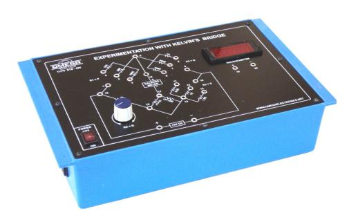
**OMEGA TYPE ETB-265 (Experimentation with Kelvin's Bridge)** is useful training product for measuring very small values of resistance, Kelvin's double bridge or Kelvin's bridge (as it is commonly known as) is a variation of wheatstone bridge and is based on the same principal. By setting the null point we can evaluate the unknown resistance.
