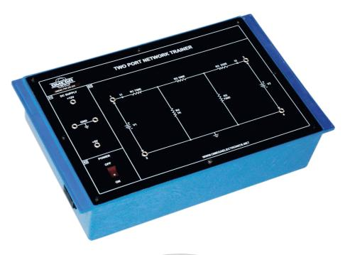
Two Port Network Trainer ETB-255 has been designed specifically for the Two Port Network analysis. This is useful for students to study the operation and behavior of any two-port network under several operating conditions. The study of twoport network is very important as they form the building block of most electrical systems.
