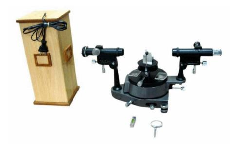
OMEGA TYPE ES-256 Experimental Set Up has been designed specifically to determine Cauchy's constant by Spectrometer. The set-up consists of Spectrometer, Mercury light source, Prism, Reading lens etc.
