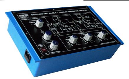
**OMEGA TYPE ETB-268** Experimental Training Board has been designed specifically for the study of Single and Two Stage R-C Coupled Transistor Amplifier.
