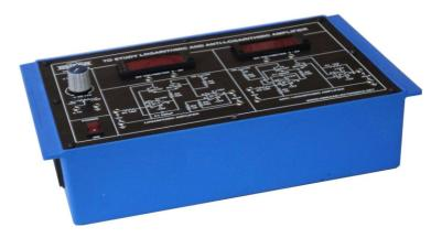
OMEGA TYPE ETB-275 Experimental Training Board has been designed specifically for the study of Temperature Compensated Logarithmic and Anti-Logarithmic Amplifier. The training board is based on temperature compensation.
