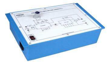
**OMEGA TYPE ETB-278** experimental training board has been designed specifically for the study of frequency multiplier using PLL (Phase Locked Loop) chip to multiply the input frequency by a factor 5. This Training board covers most of the important parameters and applications on phase locked loop (PLL) IC 565.
