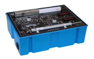
OMEGA TYPE ICT-927 Instrumentation trainer has been designed specifically for Displacement Measurement using Capacitive & Inductive Pick-Up System. The trainer consists of Linear Variable Differential Transducer (L.V.D.T.) for Capacitive Pick-Up System & Slidable Movable Capacitive Plates for Capacitive Pick-Up System. The board is absolutely self contained & requires no other apparatus. Practical experience on this set up carries great educative value for Science and Engineering Students.
