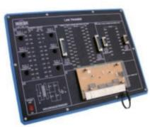
OMEGA TYPE LAN - 1011 LAN trainer is a versatile desktop system that provides hands on experimentation & understanding of local area Networks. The field being diverse, this trainer has been designed with an aim to touch upon the various aspects of LAN's such as hardware & cabling, software configuration & protocols.
