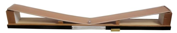
**OMEGA TYPE ES - 444** Experimental Set Up has been designed specifically to study the conservation of energy of a ball rolling down an inclined plane (using a double inclined plane).
