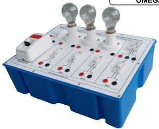
OMEGA TYPE PET - 472 Experimental Set Up has been designed specifically to assemble a household circuit comprising three bulbs, three (on/off) switches, a fuse and a power source. The set-up is absolutely selfcontained and requires no other apparatus.
