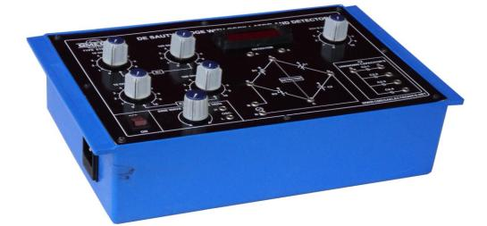
**OMEGA TYPE ETB-269** Experimental Training Board has been designed specifically for the study of De-Sauty Bridge. Using this bridge the value of unknown capacitor can be found.
