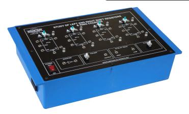
OMEGA TYPE LTB-828 Computer Logic Training Board has been designed specifically for the study of Left & Right Shift Registers & Ring Counter. This Training Board makes the student familiar about the working, practical aspect and design of the same by using inverter & J-K flip-flops. The board is absolutely self contained and requires no other apparatus.
