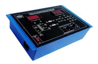
**OMEGA TYPE ETB-279** Experimental Training Board has been designed specifically to study LCR Circuits with an A.C. Source. The board is absolutely self contained and requires no other apparatus.
