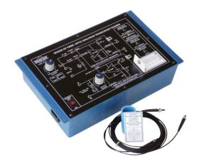
**OMEGA TYPE FO-003** Fibre-Optic Analogue Transceiver Trainer has been designed specifically for the study of a typical linear intensity modulation system for analogue signal transmission.
