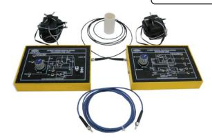
**OMEGA TYPE FO-007A&B** Laser Diode Intensity Modulation and Demodulation Trainer has been developed to conduct studies on laser diode, optical fibres and optical communication methods, by signal transmission.
