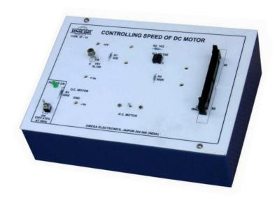
Looking to the recent requirement of Educational Institutions we have developed OMEGATYPE Controlling of speed DC Motor Interface Module which can be easily interfaced with 8085/8086 Microprocessor Trainer with the help of a flat cable connected 50 pin FRC connectors both sides. These can be also interfaced with IBM PC, XT, at with the help of a 96 BIT TTL I/O experimental interface OMEGATYPE IFB—13.
