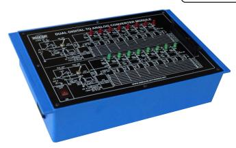
OMEGA TYPE IF-3 Dual Digital to Analog Converter Interface Module which can be easily Interfaced with 8085/8086 Microprocessor Trainer with the help of a flat cable connected 50pin FRC connectors both sides. This can be also interfaced with IBM PC, XT, AT with the help of a 96 BIT TTL I/O Experimental Interface Omega Type IFB-1.
