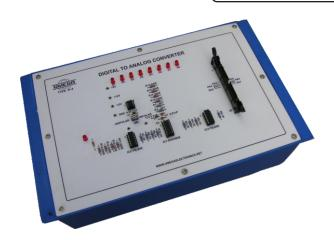
OMEGA TYPE IF- 4 Digital to Analog Converter Interface Module which can be easily Interfaced with 8085/8086 Microprocessor Trainer with the help of a flat cable connected 50 pin FRC connectors both sides. This can be also Interfaced with IBM PC, XT, AT with the help of a 96 BIT TTL I/O experimental Interface Omega Type - IFB-1.
