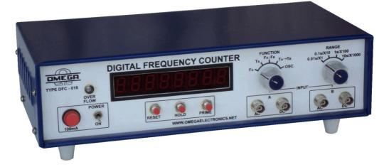
**OMEGA TYPE DFC-018** is a multifunction digital instrument. Apart from measuring frequency, it is also capable of measuring frequency ratio of two signals and their time intervals and period. This instrument is based on an advanced design which is centered around an LSI IC. This low cost equipment is rigid enough to be used as a general purpose test equipment by hobbyists, laboratories & manufacturers.
