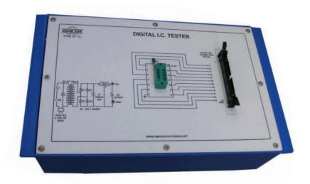
**OMEGA TYPE IF-11**, Digital IC Tester (for Quad 2-input OR / AND gate) interface module which can be easily interfaced with 8085/8086 Microprocessor trainer with the help of flat cable connected 50 pin FRC connectors both sides. This can be also interfaced with IBM PC, XT, AT with the help of 96 Bit TTL I/O experimental interface Omega type IFB-1.
