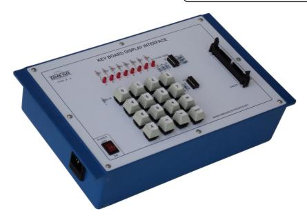
OMEGA TYPE IF- 9 Key Board Display Interface which can be easily Interfaced with 8085/8086Microprocessor Trainer with the help of a flat cable connected 50 pin FRC connectors both sides. These can be also Interfaced with IBM PC, XT, AT with the help of a 96 BIT TTL I/O experimental Interface Omega Type - IFB-1.
