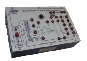
**OMEGA TYPE ETB-1** Experimental Training Board has been designed specifically for the study of Conventional D.C. High Voltage Power Supply (based on vacuum tube diodes)
