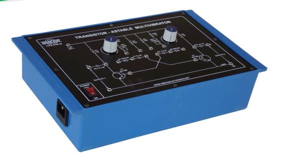
**OMEGA TYPE ETB-26** Experimental Training Board has been designed specifically for the study of Free Running (Astable) Multivibrator circuit. A free running multivibrator circuit is frequently used as a simple means of generating square wave signal.
