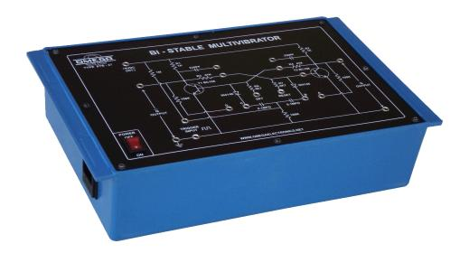
**OMEGA TYPE ETB-27**Experimental Training Board has been designed specifically for the study of Bistable Multivibrator circuit built around transistors. A bistable circuit is widely used in digital circuits.
