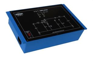
**OMEGA TYPE ETB-41** Experimental Training Board has been designed specifically for the study of FETAmplifier.
