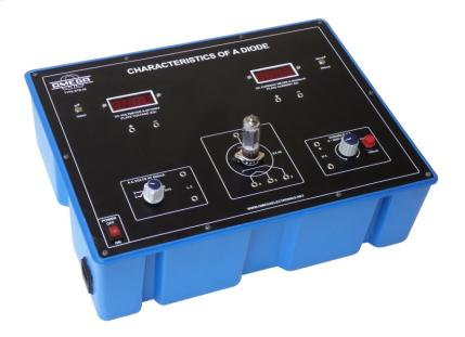
**OMEGA TYPE ETB-48** Experimental Training Board has been designed specifically for the study of the Characteristics of Vacuum Diode. The board is absolutely self contained and requires no other apparatus.
