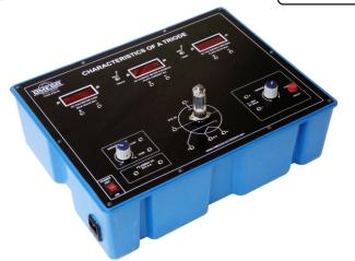
**OMEGA TYPE ETB-49** Experimental Training Board has been designed specifically to study the characteristics of Vacuum Triodes. The board is absolutely self contained and requires no other apparatus.
