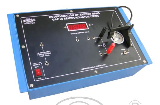
**OMEGA TYPE ETB-58** Experimental Training Board has been designed specifically for Determination of Energy Band Gap in Semiconductor (P-N Junction Diode) using Temperature dependent of reverse saturation current. The board is absolutely self contained and requires no other apparatus.
