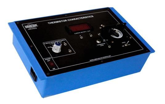
**OMEGATYPE ETB-59** Experimental Training Board has been designed specifically to study the Characteristics of a Thermistor. The board is absolutely self contained and requires no other apparatus.
